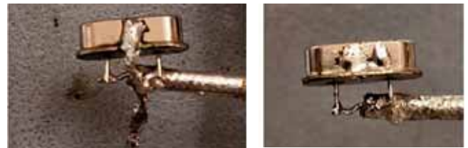
Figure 7 — Crystal connections; left grounded, right ungrounded.
