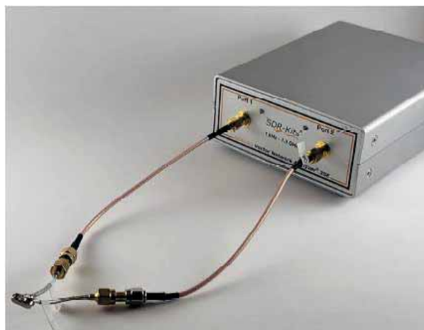
Figure 2 — VNA measurement setup.
